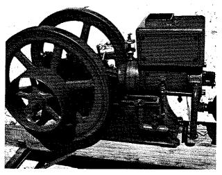
Left and below: Later Model A Economy engines featured a shallow fuel primer and choke cup, along with a raised hopper lip, indicative of ways Holm Machine changed the model to produce a better engine. Knowing these changes enables collectors to evaluate when an engine was produced.
