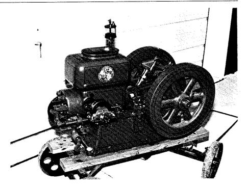
industry were the Hercules and Economy hit and miss kerosene engines. They were offered in the larger sizes in 1914 and 1915. A small cast iron gravity type gasoline tank was mounted on the off side of the engine for starting. The fuel mixer was a brass Lunkenheimer with a water and fuel adjustment valve. A three way cock was used to switch fuels. Later a three valve mixer was
