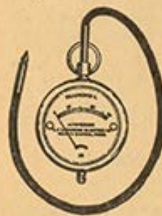
Ammeter for Testing Batteries.
