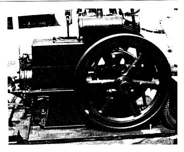
Upon compression to 450 PSI the fuel in the cup ignited, blowing the charge out into the cylinder for complete combustion. It was said that the air became "red hot."
