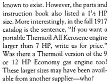
The Thermoil is not a diesel, even though many refer to them that way. The diesel patent involved injection of fuel under pressure into the cylinder in proper sequence with the compression stroke. The Hvid patent involved metering a small amount of fuel into a hole on the fuel injector valve seat. During the intake stroke this fuel valve opened and the fuel and a small charge of air was drawn into a fuel cup in the cylinder.
