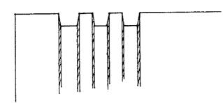
apart, cleaned up and reassembled, the compression seems to have left. If this happens, it is likely that the cylinder bore is worn out of round. Before disassembly the piston rings had worn out of round, too, but conformed to the cylinder walls. When reassembled with new or the old rings, they no longer conform to the cylinder walls and there is blow by and enough compression loss that the engine won't run or runs poorly. The solution is the same as that mentioned above.
