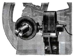
The magneto we furnish with the engine is part of the engine. It is properly adjusted and timed when it leaves the factory and should not be
